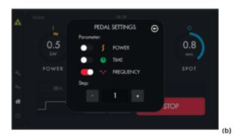
By clicking on the footswitch icon, the user opens a dialog box where it is possible to select both the desired parameter (power, frequency, or time) and the increment factor.
